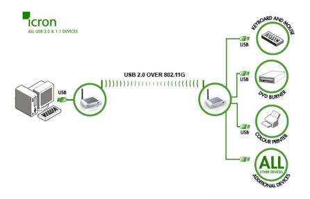
The LEX unit and REX unit of this WiRanger are "Paired" at the factory so that they will only communicate with each other, even if other WiRanger's are installed near by.
